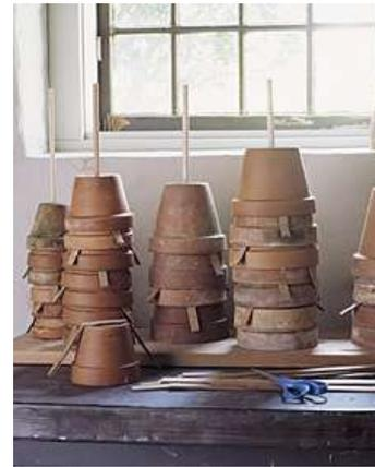
Secure stacks of terra-cotta pots so they don't stick together or tilt dangerously. Drill 1/2-inch holes, spaced to fit pot diameters, through a 1-by-10 (atop scrap lumber). Apply wood glue to bottom inch of 1/2-inch dowels no longer than 18 inches. Insert in holes, squaring with base; let dry overnight. Sandwich 1-by-12-inch corrugated-cardboard strips between pots on rack.
